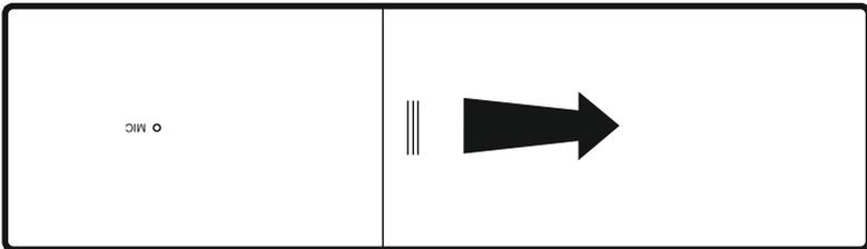
\* You can teach the Power button from the original remote control. 1) Hold the Power button for 3 sec (you can see the red blinking indication on the smart remote). 2) Line up smart remote and original remote head-to-head. 3) Push a button on the original remote.
